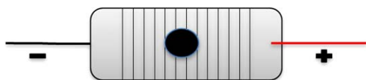
Figure 3. Diagram illustrating direction of fiber alignment, droplet location and contact points for application of electric field (note that image is not drawn to scale). [Color figure can be viewed in the online issue, which is available at wileyonlinelibrary.com .]
